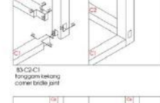
B3-C2, C1 tanggam rengang corner blade joint
